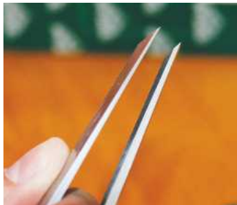
▲ The 6mm chisel (right) has slightly thicker lands than the rest of the set
